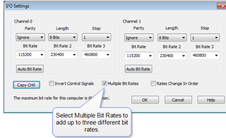
Figure 3.1 - HSU I/O Settings - Multiple Bit Rates
