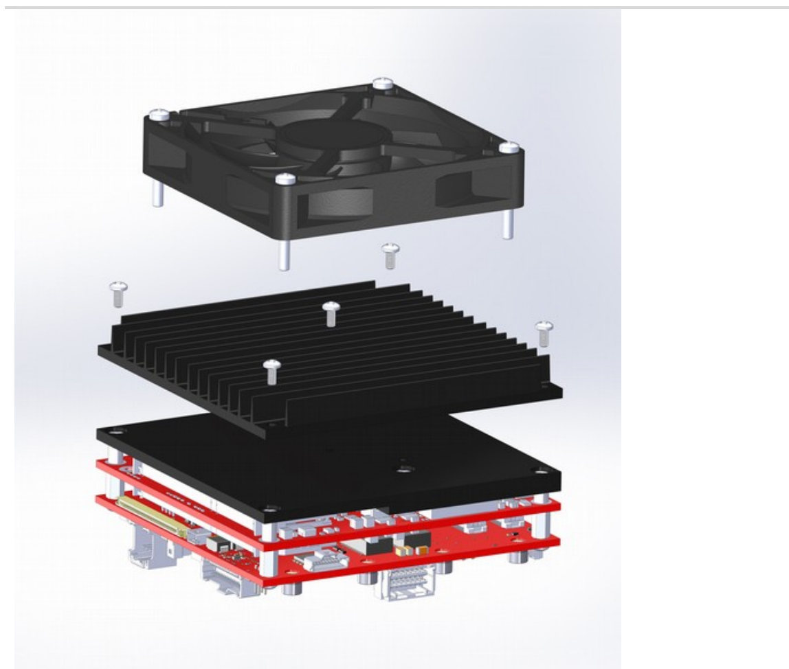
Figure 32. Installing the Heat Sink Fan
